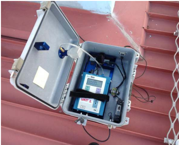
Figure 8: DustTrak monitor atop Council's Administration Building (photo N Smith, ARC)
